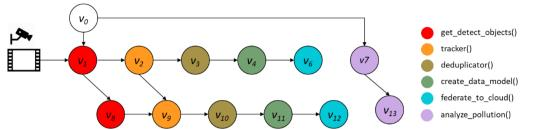
Figure 4. COMPSs DAG for two iterations of the workflow for a single camera source
