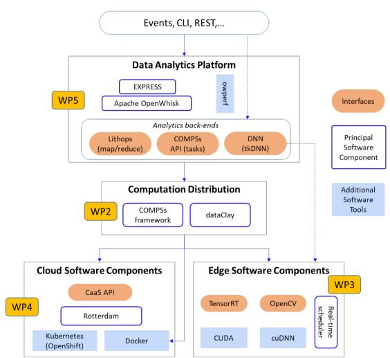
Figure 1. The final release of the CLASS Software Architecture Ecosystem
