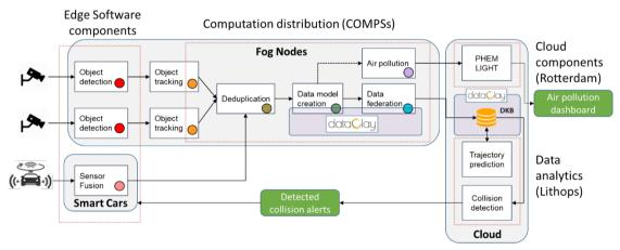
*Figure 6. Description of the execution of the collision detection and air pollution estimation applications over the CLASS software architecture*
