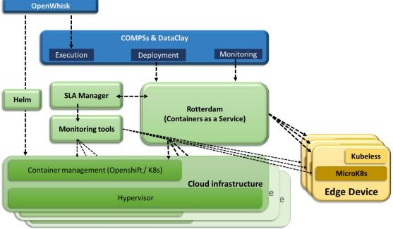
*Figure 2 – Cloud computing platform in the context of the CLASS architecture*
