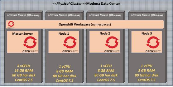
Figure 7 – Modena Data Center deployment
